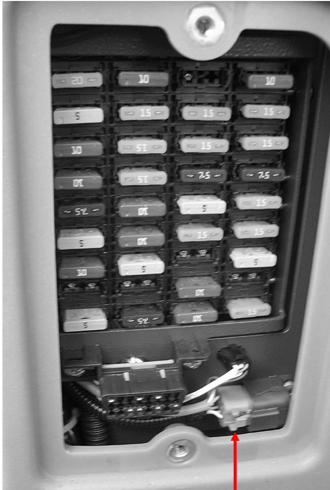
X59 Steckdose 6pol. Diagnose Yanmar X59 Diagnosis Yanmar, socket (plug) 6 pole
